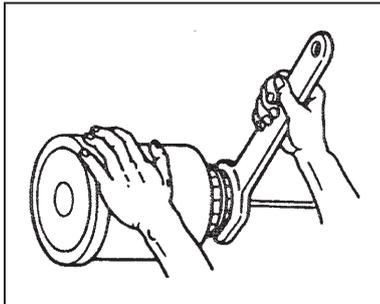
3. Install the level sensor into the new fuel filter with a wrench.
