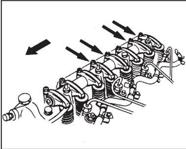
4. Turn the crankshaft one full turn (360 degrees) and adjust the clearances of the valves indicated by arrows.
