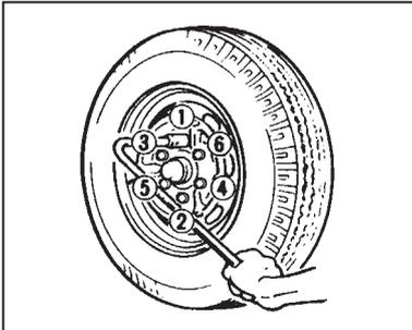
3. With the wheel wrench, tighten the wheel nuts in sequence as shown in the figure.
