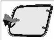
5. To lock the window in closed position, press the handle till the click sound is heard.
