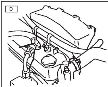
Next fill the engine crankcase from the filler port with new engine oil of the specified grade.
