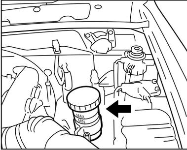
5. Bring the steering wheel to the straight-ahead position, stop the engine, and check that the level of fluid in the fluid reservoir does not rise. If the fluid level rises sharply, air is not completely removed from the system and the operations outlined under step 4 must be repeated.
