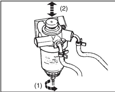
3. After draining, securely tighten the drain plug (1) by turning it clockwise and operate the hand pump up and down (2) several times.
