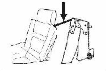
6. Attach the band (with hook) provided below the third seat to clasp on to the head rest of the second seat back.
