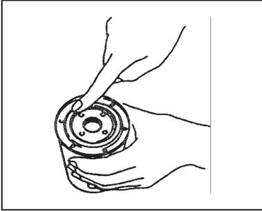
4. Wipe the fitting face of the filter cover clean with a rag, so that the new fuel filter can be seated properly.
