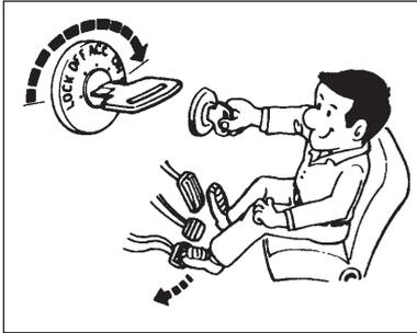
2. Crank up the engine by turning the starter switch key fully clockwise. Release the key as soon as the engine starts. The key will return automatically to "ON."
