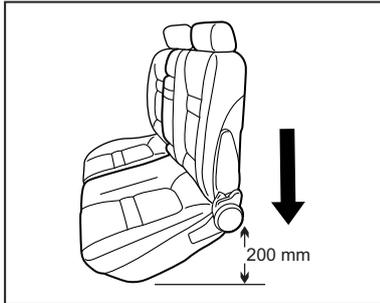
3. Drop the seat assembly from height of about 200mm with backrest straight.
