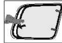
4. For closing the window, un secure the handle and pull the handle inwards to close the window.
