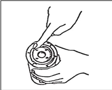
3. Lightly oil the O-ring and turn the oil filter until the sealing face is fitted against the O-ring. Turn one full turn further with the filter wrench.
