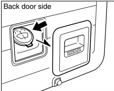
Insert the lower portion of the cover first while re-fitting
