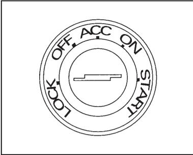
“START” : Turning the key to this position will start the engine.
