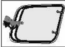
3. To hold the window in the open position, secure the handle in lock position by pushing it in the direction as shown.
