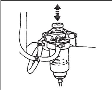
6. Operate the priming pump on the water separator several times to bleed fuel system air.
