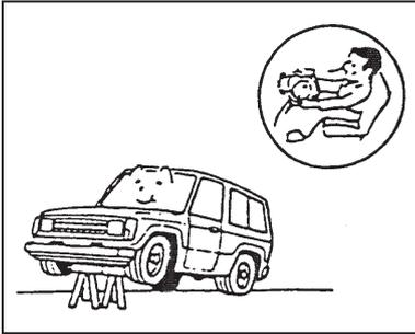
2. With the engine stationary, turn the steering wheel fully in both directions several times.
