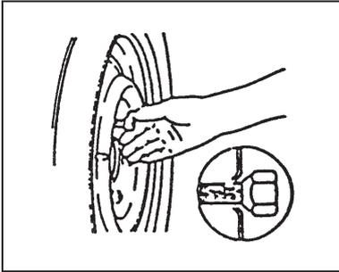
2. Install and semi-tighten the wheel nuts and lower the wheel to the ground.
