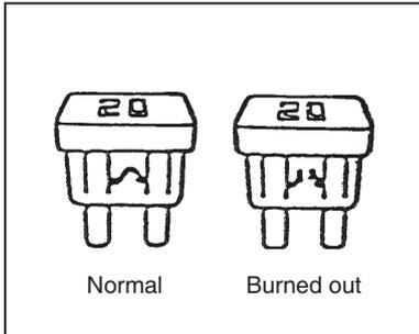
The drawing at the left illustrates a burned out fuse.
