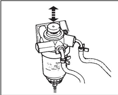
1. Operate the hand pump on the water separator to bleed fuel system air into the injection pump.
