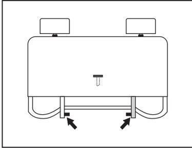
4. Pull the seat latch lever towards your side to detach the seat latch.
