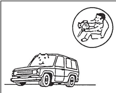
3. With the engine idling turn the steering wheel fully several times in both directions
