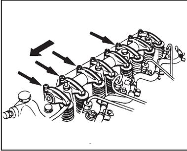
3. Adjust the clearance of the valves indicated by arrows.
