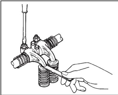
2. Adjust the valve clearances in the following manner using a feeler gauge.
