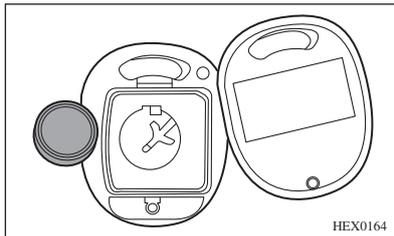
If the LED fails to illuminate or if the range is noticeably diminished, it is an indication that a new battery is needed.
