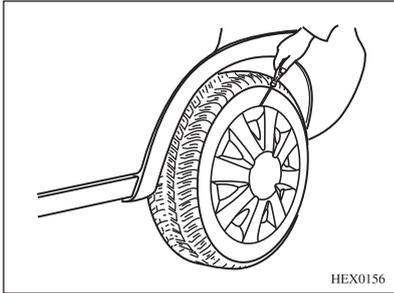
6. Use a screwdriver to remove the wheel cover (if equipped).
