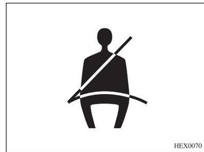
When the ignition switch is ON, the safety belt warning light will illuminate briefly. This means that the system is carrying out a self-test.
