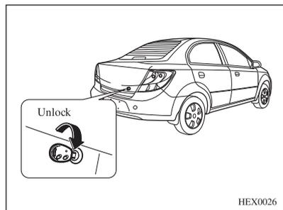
Insert the key and turn it clockwise to unlock the trunk. Lift the trunk.
