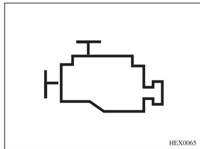
After the ignition switch is turned ON and before the engine is started, the indicator light will illuminate.
