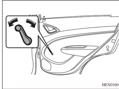
To raise or lower the windows, turn the window regulator handle on the door panel.
