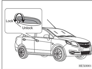
Use your key to unlock the vehicle from the driver door. Use the same key to unlock the rear compartment.
