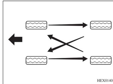
Front tires and rear tires have different working conditions, and therefore they wear out at different rates.
