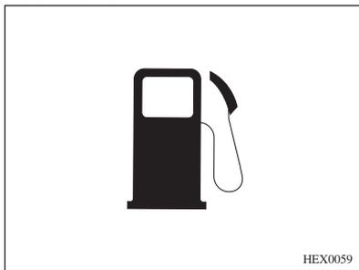
This light comes on when the fuel tank is low on fuel. When fuel is added, the light should go off. If it does not, have the vehicle serviced.
