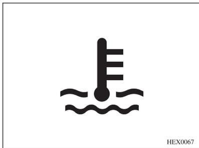
The engine coolant temperature warning light comes on briefly when the ignition is turned ON. This shows that the system is doing a self-test and the indicator light bulb is working correctly. If the system is working normally the indicator light then goes off.
