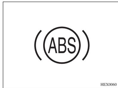
If the vehicle is equipped with ABS, when the ignition switch is turned ON, the ABS warning light will illuminate for a moment. This shows that the system is doing a self-test and the indicator light bulb is working correctly. This warning light should go off after a few seconds.
