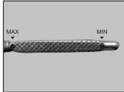
6. Check the oil level on the dipstick. Make sure the oil is not contaminated.
