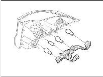
4. Push in and turn the bulb counter-clockwise to remove it from the socket.
