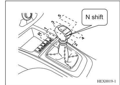
To change gears, fully depress the clutch pedal, move the gearshift lever into gear, and slowly release the clutch pedal.
