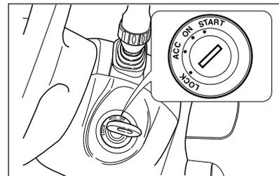
Located to the right side of steering column, the ignition switch has the following positions: LOCK, ACC, ON, and START.
