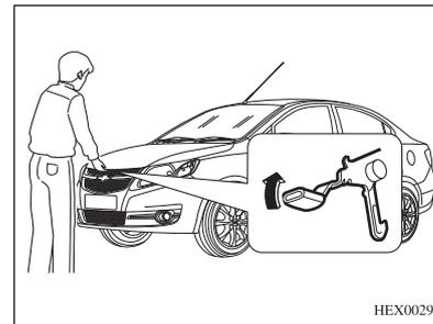
2. Reach under the front edge of the hood and lift the hood release handle.
