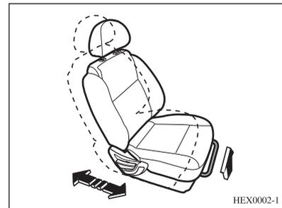
Pull the handle up and slide the seat forward or backward to an appropriate position, then release the handle. Slide the seat forward and backward to ensure it is locked in the appropriate position.
