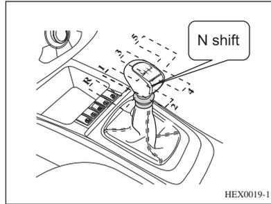
To change gears, fully depress the clutch pedal, move the gearshift lever into gear according to the gear position marked on gear knob and slowly release the clutch.
