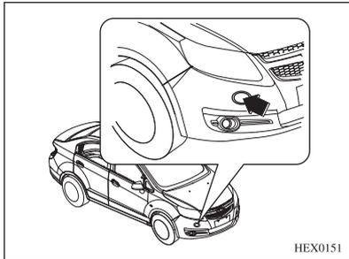
There is a round cover at the right hand side of the front bumper. A fixing hole for hook installation can be found after you open the cover by pressing it on the driver side, as indicated by the arrow in above diagram. The hook is stored in the tool bag in the rear compartment.
