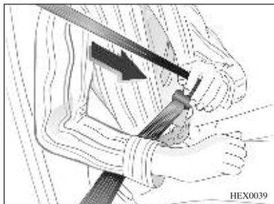
Pull the seat belt out of the retractor, guide it across the body without any twists, and then buckle the belt.
