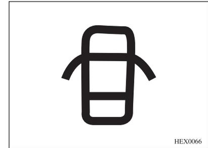
This light comes on when a door is open or not securely latched. Before driving check that all doors are properly closed.
