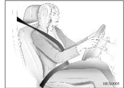
Pull out the safety belt strap and insert it into the buckle. The belt strap must not be twisted and must be worn fitted closely against the body. The seatback should not be excessively reclined.
