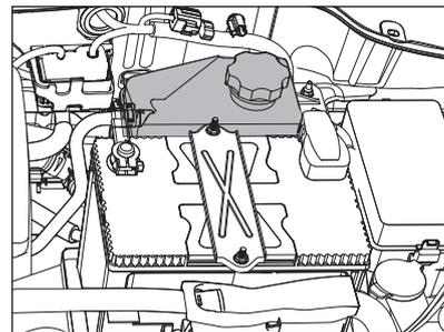
If the coolant level falls below the MIN mark, refill the reservoir with General Motors India Pvt. Ltd. recommended coolant available with your CHEVROLET retailer, but only when the engine is cool. In order to protect your vehicle in extremely cold weather, use GMI approved coolant.
