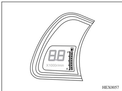
Displays the fuel level in the fuel tank. If the fuel level in the fuel tank is too low, the control indicator light will illuminate. Please refuel immediately.
