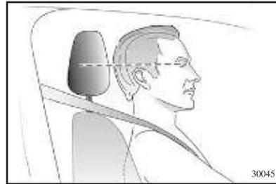
The center of the head restraint should be at eye level of the occupants. If this is not possible for extremely tall people, set to highest position, and set to lowest position for short people.
