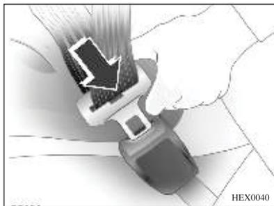
Loose or thick clothes will obstruct the position of the safety belt over the body. Do not place anything (e.g. a handbag or a mobile phone) between the safety belt and your body.
