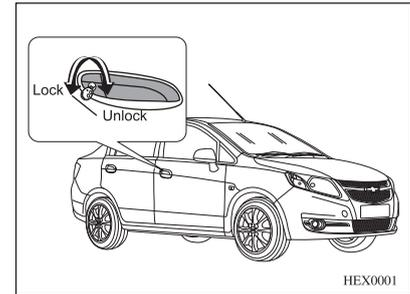
Driver door lock - Turn key clockwise to unlock and counter clockwise to lock the driver door.
