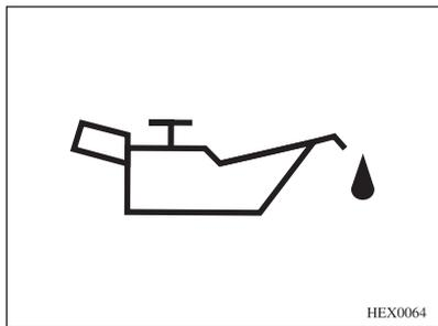
After the ignition switch is turned ON and before the engine is started, the warning light will illuminate. This shows that the indicator light bulb is working correctly.
