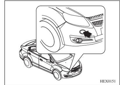
If towing service is not available in an emergency, the vehicle may be towed temporarily by securing a cable to the front hook under the vehicle. When the front hook is used in towing, you can only use a tow rope, not a rigid towing bar.
