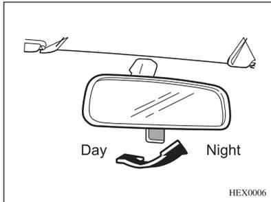
The interior rear view mirror can be adjusted manually.
