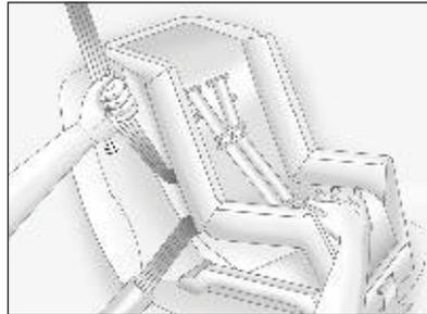
4. To tighten the belt, push down on the child restraint, pull the shoulder portion of the belt to tighten the lap portion of the belt and feed the shoulder belt back into the retractor. When installing a forward-facing child restraint, it may be helpful to use your knee to push down on the
