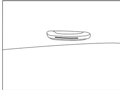
Your vehicle has assist grips above the front seat passenger's door and the rear doors.
