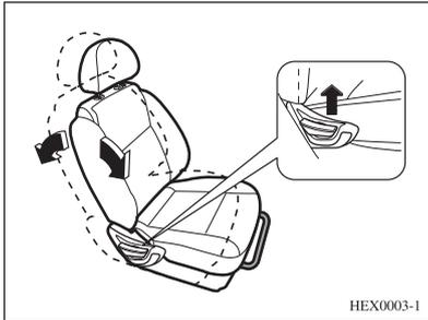
Lift the lever, adjust the seatback to an appropriate position, then release the lever.
