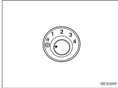
You can control the amount of airflow by turning the fan speed control knob. Turn the knob clockwise to increase fan speed, or counterclockwise to decrease fan speed.
