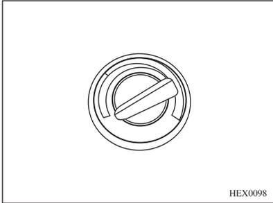
The temperature control selector controls the temperature of air flowing out of the vents.
