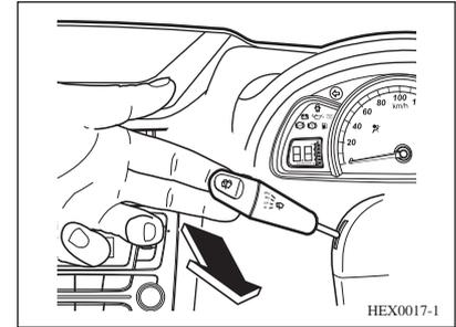
Pull the control lever towards you, as shown in the picture to wash the windshield.
