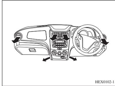
Directs air flow in two ways. Half of the air through the floor vents and the remaining through the center and side vents.
