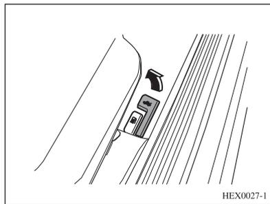
You can open the trunk by pulling the trunk release lever which is mounted on the floor to the right of the driver seat.
