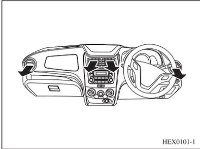
This mode directs airflow through the center vents and side vents.
