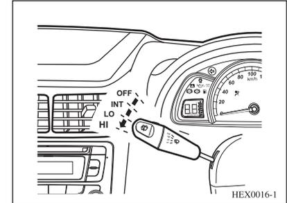
To use the windshield wipers, first turn ON the ignition switch, then push the windshield washer/wiper lever downwards.
