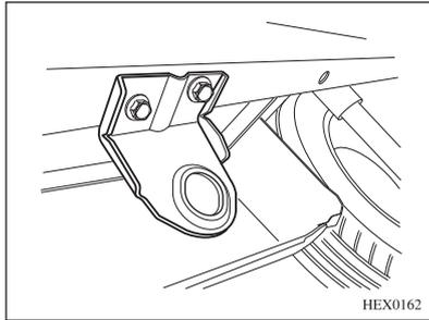
The towing hook for shipping is located below the left part of the rear bumper on the vehicle body floor, and is used when this vehicle is shipped.
