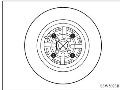
16. Tighten the wheel nuts to 130 Nm, in a diagonal pattern.
