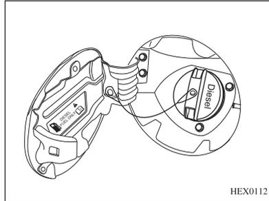
3. Turn the fuel filler cap counter-clockwise. If there is a hissing sound, wait until it stops before unscrewing the cap. The fuel filler door is in the left rear quarter panel.
