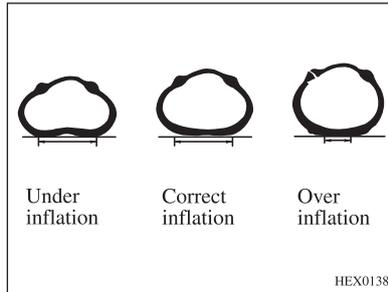
The tire pressure should comply with the specifications in this Manual to ensure optimal ride comfort, safety and performance. The tire pressure label is on the driver's door frame.
