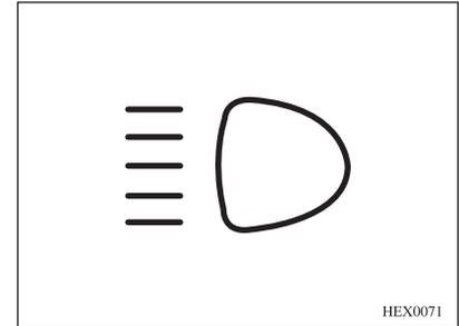
The high-beam indicator comes on when the high-beam headlamps are in use and during headlamp flash.
