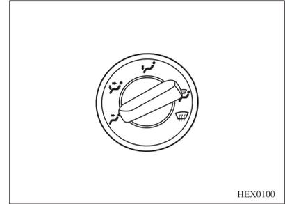
Turn the knob to the desired mode according to the desired airflow direction.
