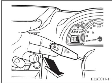
To spray washer-fluid onto the windshield:
