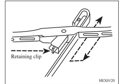
1. Press and hold the blade retaining clip.
