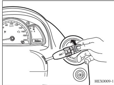
To turn the headlamps, tail lamps or parking lights on or off, turn the end of the combination switch lever.
