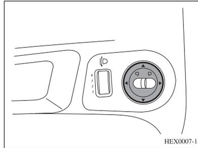
The exterior rear view mirrors can be adjusted by using the mirror switch that is located on the instrument panel to the right side of the steering wheel. The ignition switch must be at ACC or ON position for this feature to work.
