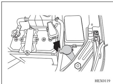
Before you drive, make sure the windshield washer fluid reservoir is at the appropriate level and filled with the correct solution.
