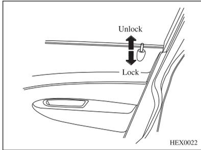
To lock the door from inside, press the door lock knob.
