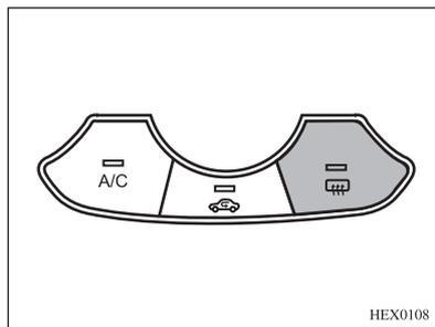
To turn on the defroster, switch ON the ignition and then press the rear window defroster button. The indicator light on the button will turn on.
