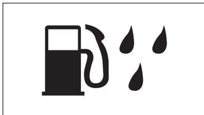
Illuminates, when the water level, in the water separator (separated from the diesel fuel) reaches to the maximum.
