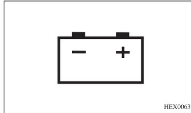
The charging system light comes on briefly when the ignition is turned ON, but the engine is not running, as a check to show the light is working. The light turns off when the engine is started. If it does not, have the vehicle serviced by your CHEVROLET retailer. If the light stays on, or comes on while driving, there could be a problem with the electrical charging system. Have it checked by your CHEVROLET retailer. Driving while this light is on could drain the battery.
