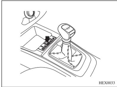
The power window lockout button can lock out the rear window switches. The rear windows can only be operated by the front switches after this button is locked.
