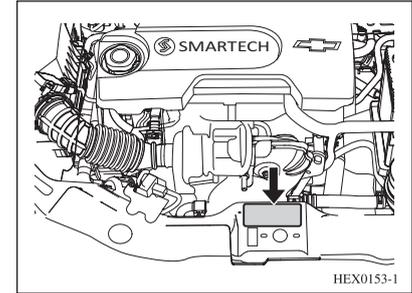
The vehicle identification number (VIN) plate is attached to the top of the front end upper panel.
