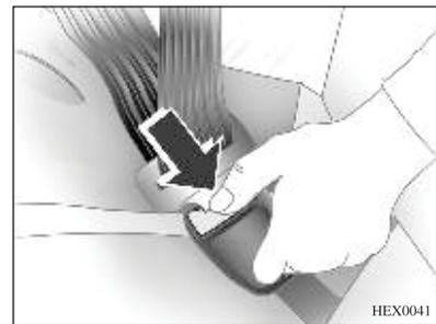
To release the safety belt, push the red button on the buckle.
