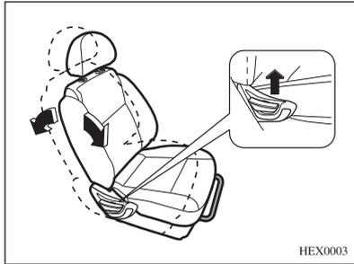
Lift the control lever, adjust the seatback to an appropriate position, and then release the control lever.
