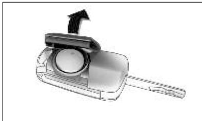
If the range is noticeably diminished, it is an indication that a new battery is needed.
