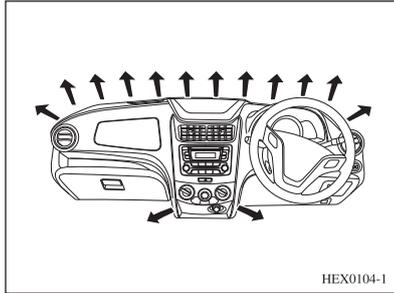
This mode directs airflow through the windshield defroster vent, front window vents, floor vents and side vents.
