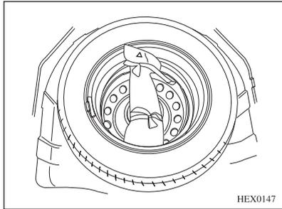
After the tool bag is packed, place the warning triangle properly according to the picture. Warning triangle is provided at the time of vehicle delivery.
