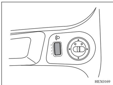
The headlamp range adjustment knob is located at the right of instrument panel.
