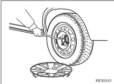
7. Use the wheel wrench to loosen the wheel nuts by a half to one turn each. Do not loosen them completely.
