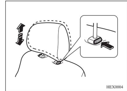
When adjusting the head restraint upwards, pull it up to the appropriate position and then secure. Press the release button to remove the head restraint out.
