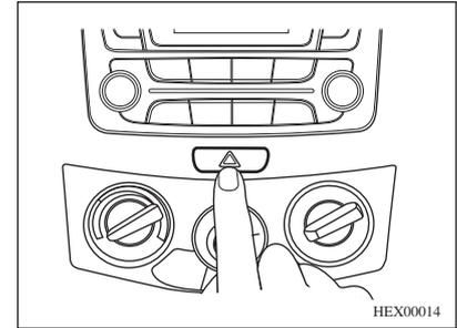
Press the  $\triangle$  switch to turn on or turn off the hazard warning flashers.
