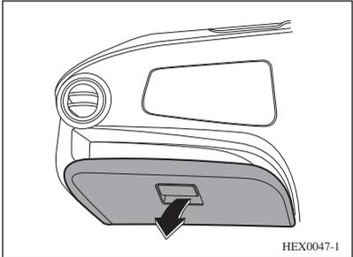
Glove box can be opened by pulling the handle.
