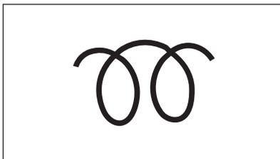
Illuminates when the ignition is ON and stays on for a short time or may go off right away. The waiting time will vary according to the engine coolant temperature.
