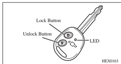
Remote Keyless Entry allows you to lock and unlock doors using the transmitter within valid operating range. The LED on the transmitter flashes to indicate an effective operation.
