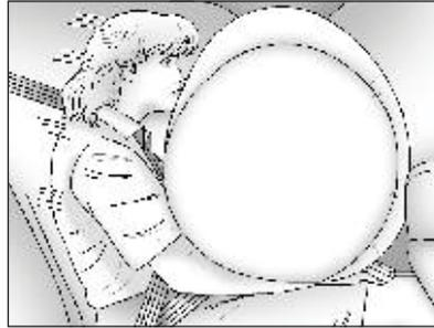
The outboard front passenger frontal airbag is in the instrument panel on the passenger side.
