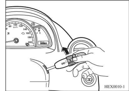
While the headlights are on parking light or low beam position, turn the ring in the middle of the combination switch lever to ON to turn on the front fog lights. Turn the ring to OFF position to turn off the front fog lights.
