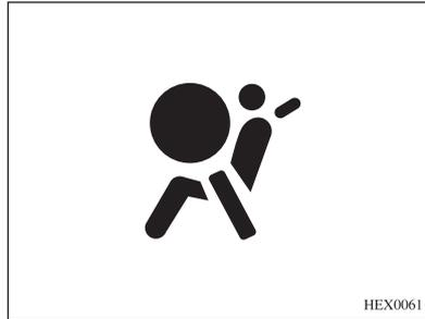
When the ignition switch is turned ON, the airbag warning light will illuminate briefly. This shows that the indicator light bulb and airbag systems are functioning properly.
