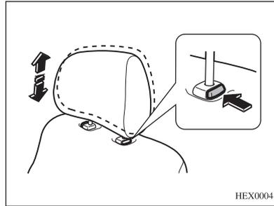
When adjusting the head restraint upwards, pull it up to the appropriate position and then fix. To pull out a head restraint completely, press the release button and take out the head restraint.
