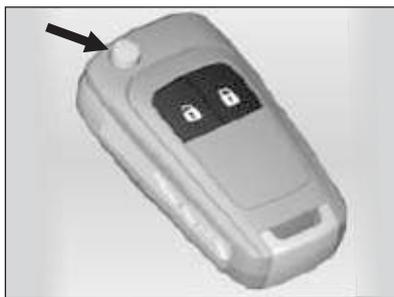
Press the button indicated by the arrow in the picture below to unfold the key.
