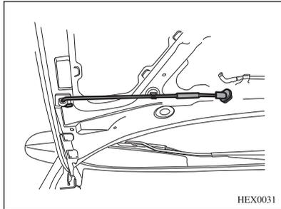
1. While holding the hood to prevent it from falling, remove the hood support rod from the recess and press it firmly into the fixing clip.
