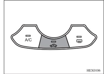
Press this button when driving in dusty conditions, to keep vehicle exhaust or smoke out, or when quick heating or cooling is desired. The indicator light on the button will illuminate and air recirculation will start.
