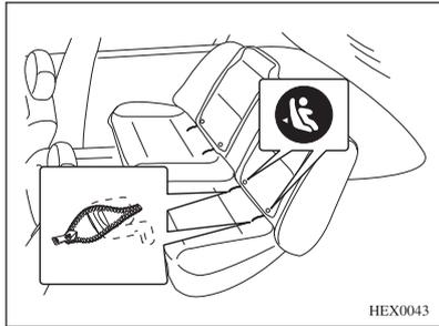
2. Clear all items off the seat. Move safety belts and safety belt buckles away from the lower anchors so they do not interfere with proper latching.
