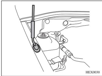
3. Release the hood support rod from the fixing clip.
