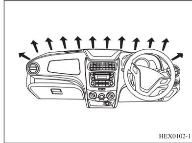
Air flows through windshield and front window defroster vents as well as side vents.
