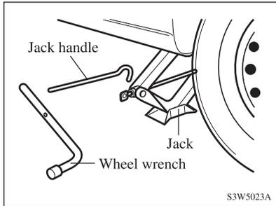
10. When rotating the jack handle, make sure the jack base is in contact with ground and directly under the notch on the lugs.
