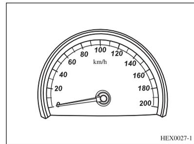
The speedometer shows the vehicle's speed in kilometer per hour (km/h).
