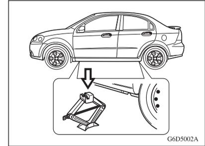
9. The jack should be placed at a jacking point nearest to the tire you want to change. The jack lift head (indicated by the arrow) should be placed around the vertical lugs and inserted into the notch of the lugs.
