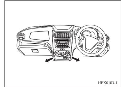
Most of the air flows through the floor vents, with a small amount of air through the windshield and front window defroster vents as well as side vents.
