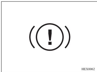
When the ignition switch is turned ON and before the engine is started, the brake system warning light will illuminate.
