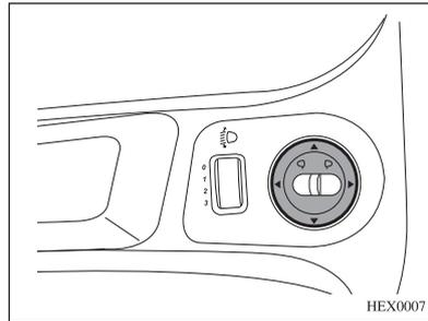
Select the corresponding exterior rear view mirror and adjust its position.
