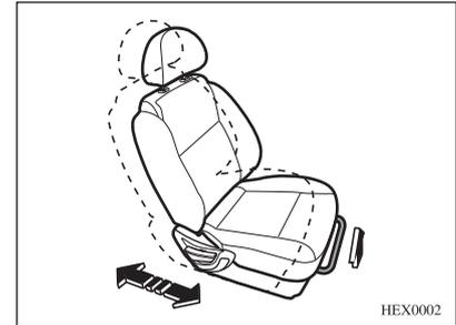
Lift the adjustment lever, slide the seat back and forth as required. Release the lever.
